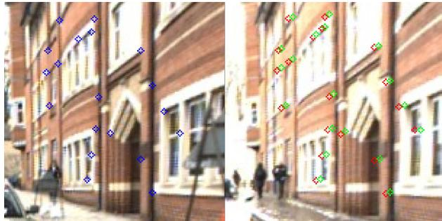
Figure 1: **Feature matching accuracy.** Corresponding sparse-to-dense feature matches between reference and query images. The matched detections on the query image (red) are a few pixels off from the points detected in the reference image (blue). Our pose refinement moves the points closer to their ground truth reprojections (blue), resulting in more accurate pose.
