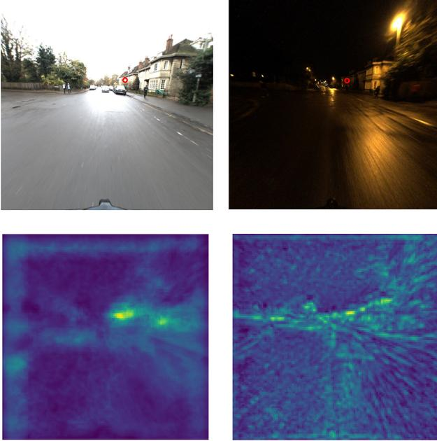
Figure 2: **Correlation map for hypercolumn matching.** First row depicts a reference (left) and a query image (right) with corresponding matches in red. Second row shows the correlation map from a reference feature to the dense query feature map. Correlation of the deeper layers of the network are shown left, while the right image shows correlations of the earlier layers of the network.
